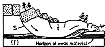
旋轉破壞 (Rotational failure)
